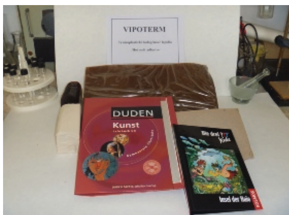
FIGURE 7.5 Thermoplastic collagen adhesive used for gluing of book hard covers.
