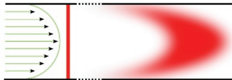
FIGURE 20.2 Schematic representation of the Taylor dispersion technique. 6
